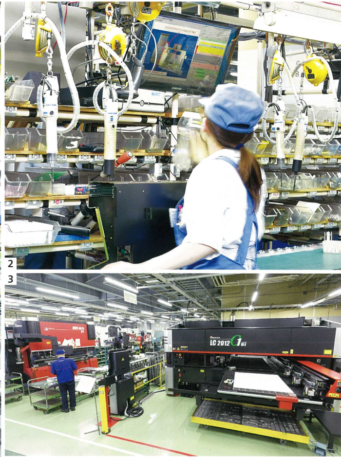
1) Units assembling line 2) The digital Yatai manufacturing system based on the internally developed digital procedure adopted for the units assembling line 3) Sheet metal process at the “Processing Technology Center” in the Shiga factory. The center produces core parts, creates development prototypes, and manufactures parts required after delivery
